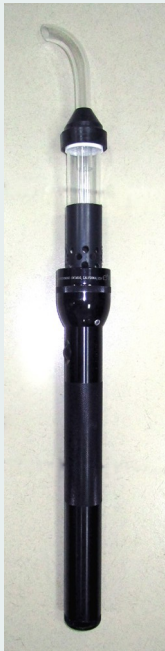
Figure 3.2: Battery operated aspirator
