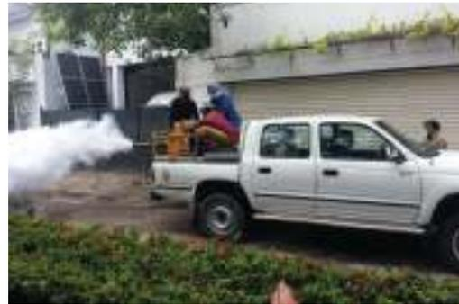
**Fig. 5.14 Thermal fogging using vehicle mounted fogging machine**
