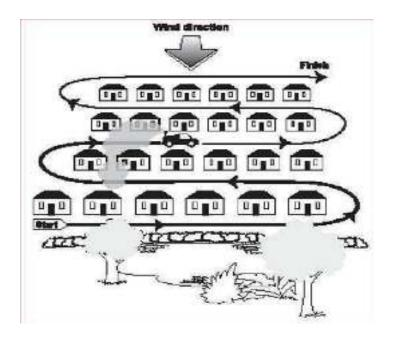
Fig.5.16. Possible movement of a vehicle mounted thermal fogging machine
